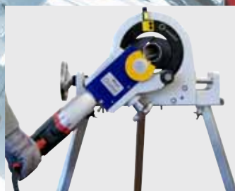
Cutting thin-walled stainless-steel tubes and elbows
