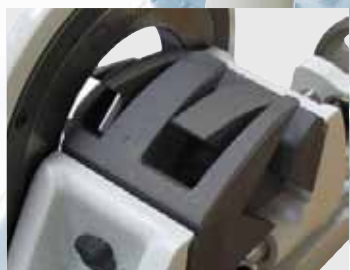
Deformation-free clamping of thin-walled tubes
