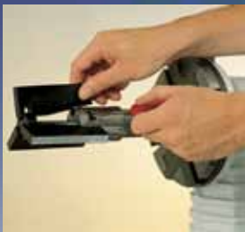
Fast adjustment of the pipe dimension
