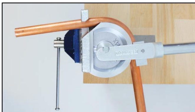
Tube bender No 30 22 mm fixed in a vice
