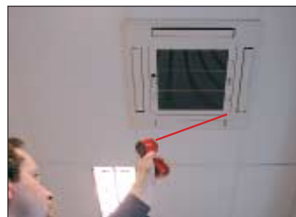
Measuring efficiency of heat dissipation in air ducts to reveal and locate thermal losses in the flow system.
