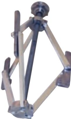
Aids in fast, accurate pipe construction with self-determining flange aligning tool. Inserts easily into pipe, centers snugly against the inside pipe diameter and automatically aligns with the pipe axis. Quickly adjustable for all types of flanges or pipe sizes ranging from 3" to 12" diameter.
