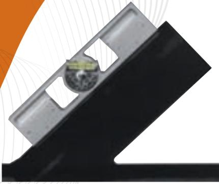
A lightweight, easy to use tool for determining angles. Unit is ideal for the pipe fitter, welder, jig builder or anyone who has to determine angles or do setup work. Includes two cast-in 25-pound pull magnets that hold securely to any steel surface. Unit has a 360° adjustable DSL with two 90° quadrants graduated in 2-1/2° increments. Cast in tables are used to convert degree-of-angle to rise-in-inches-per-foot or millimeters-per-meter. A groove on the bottom edge permits use on a small pipe.
