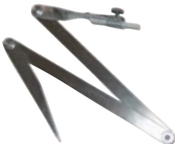
Models available in four sizes for scribing circles up to 80" in diameter. Folding type design--three smallest models will fit conveniently into a shirt pocket. Sturdy friction joints maintain rigidity and accuracy, and are made from lightweight, rustproof aluminum for long wear. Soapstone crayon is included. The scribe holder will accept round, square or flat soap stone crayon, pencil or steel point scribe.
