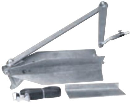
Developed for use in the layout of large diameter pipe, from 8" to 48" and structural seal joints, of the same size pipe. Comes complete with a durable web strap (included) to help hold the unit in place during layout. Built-in adjustable dial set level (DSL) ensures accurate center-line location. A soapstone crayon is included.
