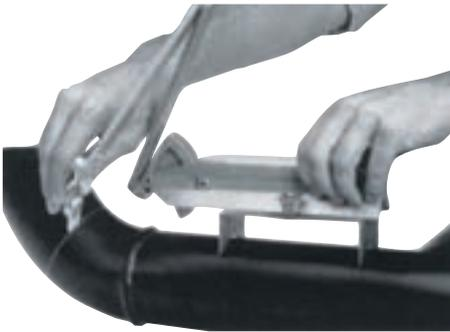
Designed for use with the Standard and Jumbo Contour Markers, the adaptor simplifies handling and increases layout flexibility. Permits use of all four sides of the Contour Marker and allows marking on small diameter pipe, over nipples, old weld or on wrapped pipe. Also provides layouts with compound angles. Using a single setting, or any degree of take-off on elbows and turns up to 90°.
