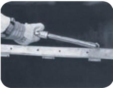
Designed for use with a burning torch or plasma cutter as straight edge, the Burning Guide is cast of strong, durable material to withstand heat spatter. Tool's base has three 30-pound pull cast-in magnets for use in any position.
