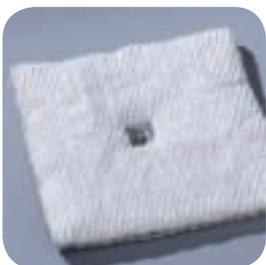
These flexible pads are made from special non-asbestos, resilient, high temperature materials. Non-combustible and chemically inert, they provide temporary insulation of welds during stress relieving of large diameter piping, ducts, vessels, or tanks. Available in 12", 24" or 48" widths and 1", 1.5", and 2" thicknesses.
